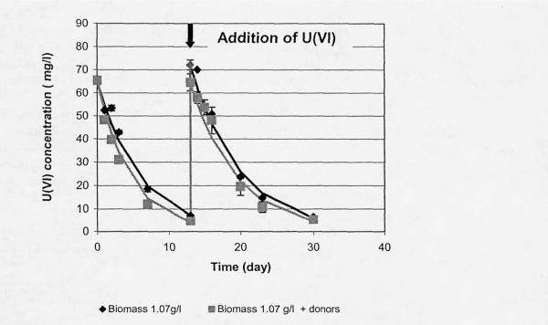
FIGURE 3 Time course of U(VI) reduction by sequential spiking U(VI). The initial biomass concentration was 1.07 g VSS/L. Uranyl nitrate was added to test bottles on day 13.
