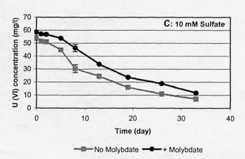
FIGURE 5 Effect of addition of Na<sub>2</sub>MoO<sub>4</sub> (10 mM) on U(VI) reduction in the presence of various initial sulfate concentrations (2, 5, and 10 mM).
