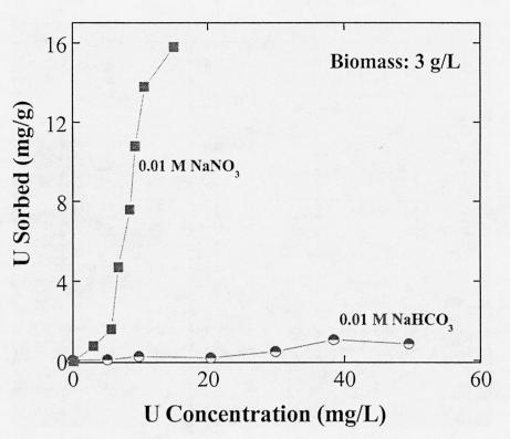
FIGURE 2 U(VI) sorption or precipitation on FBR biomass in 0.01 M NaHCO3 or NaNO3 background electrolyte solution.
