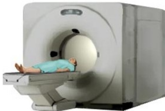
Figure 7: The magnetic field in MRI is produced by a solenoid.
