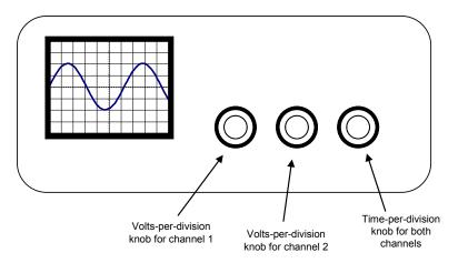
The most important idea for a novice to learn is that the oscilloscope is a measuring device. It does not generate the signal being observed on the screen, and no combination of button-presses and knob-turns ever changes the signal. The *appearance* of the signal on the screen might change, but this is only because the vertical scale and/or horizontal scale or some other display setting has changed, not because the actual signal has changed.
