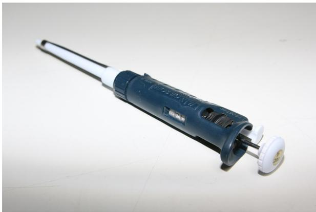
Air displacement means that upon depressing the white knob or plunger with the thumb, air is pushed out of the barrel and subsequently, out of the disposable tip attached to the end of the barrel. Pushing should cease when distinct resistance is felt. This is described as the “first stop”. Air should be pushed out of the tip prior to immersion in the source solution.
